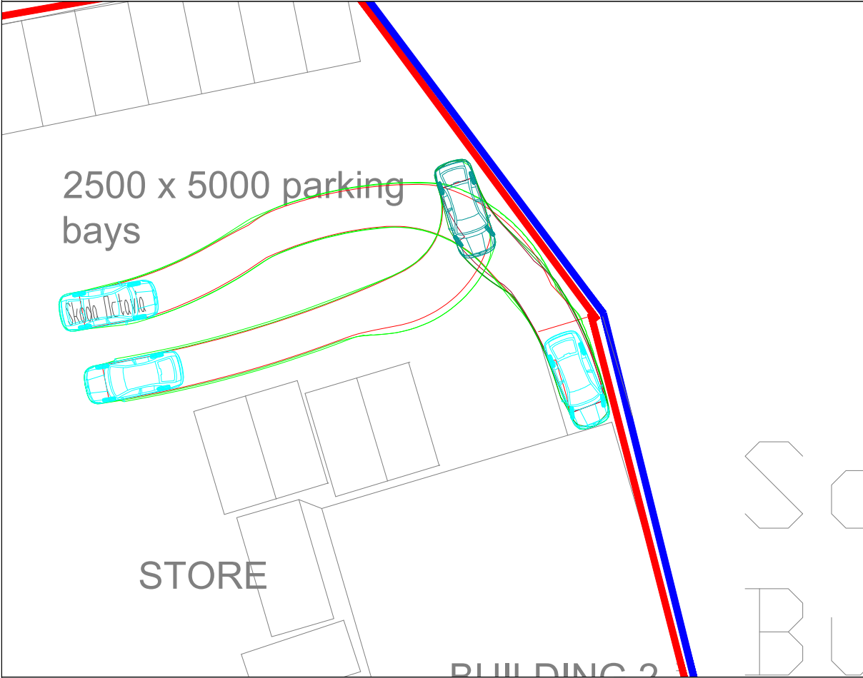
CAR PARK TRACKING 3
