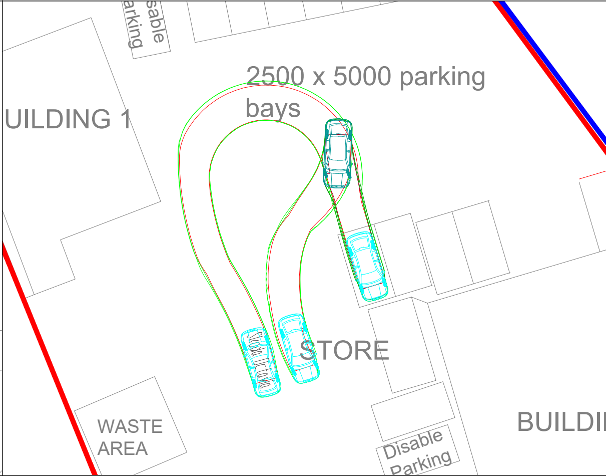
CAR PARK TRACKING 4
