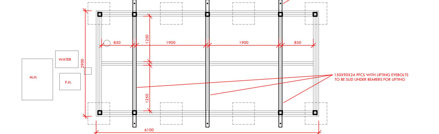
FLOOR STRUCTURE & LIFTING PLAN
