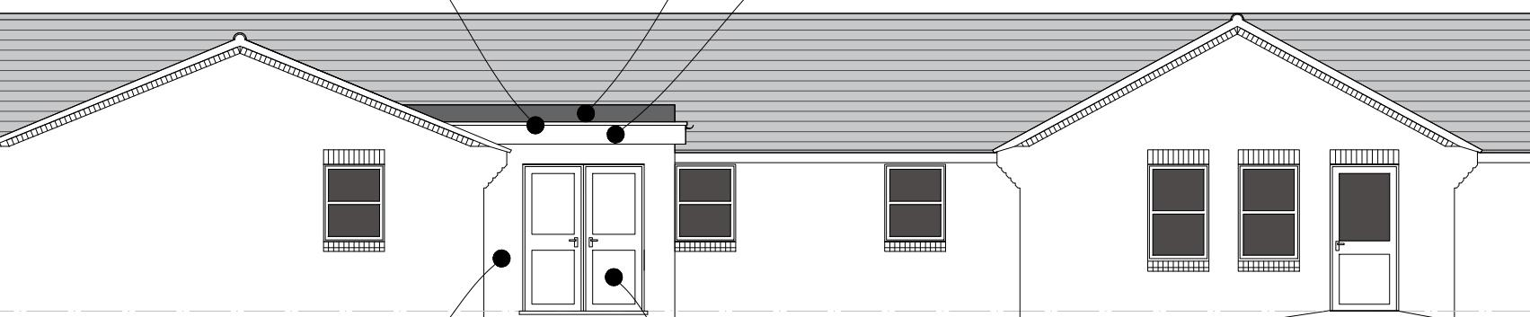
Proposed external walls are red brick laid in stretcher bond.
