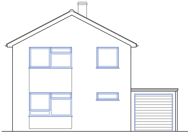
EXISTING FRONT ELEVATION
