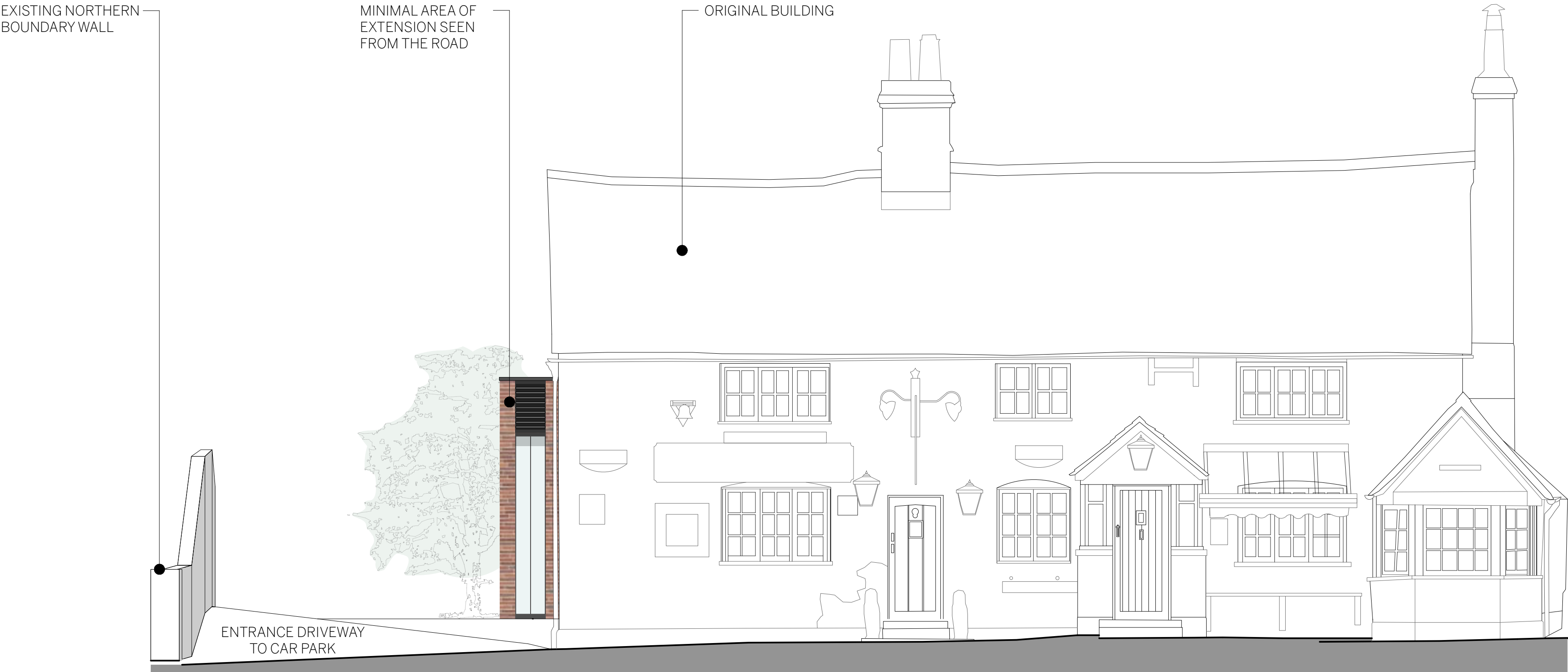
PROPOSED WEST ELEVATION (PERGOLA REMOVED)
